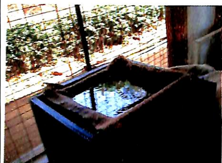
Above : Charcoal cooler with water held on top of the trough
