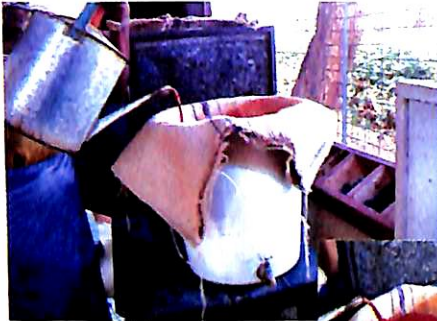
Left : Typical mud water poured into the water filter
